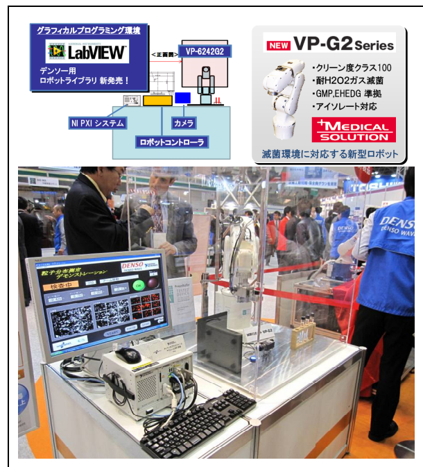
圖三 Control your DENSO Robot with NI LabVIEW and NI PXI 會場展示照片
